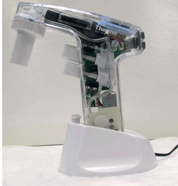
FIGURE 9-5 A pipette filler for use with serological pipettes ranging in size from 1 mL to 100 mL.
