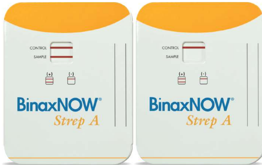
FIGURE 20-13 BinaxNOW lateral flow assay. The BinaxNOW Strep A Test immunochromatographic assay for the qualitative detection of Streptococcus pyogenes Group A antigen from throat swab specimens. To perform the test, a throat swab is inserted into the test card. Extraction reagents are added from dropper bottles. The test card is closed to bring the extracted sample in contact with the test strip. Strep A antigen captured by immobilized anti-strep A reacts to bind conjugated antibody. Immobilized species antibody captures the second visualizing conjugate. The test is interpreted by the presence or absence of visually detectable pink-to-purple colored lines. A positive result is indicated by production of both a sample line and a control line (shown on left), whereas a negative assay will produce only the control line (shown on right). ( BinaxNOW is a trademark of the Alere Scarborough, Inc. Used with permission. )
