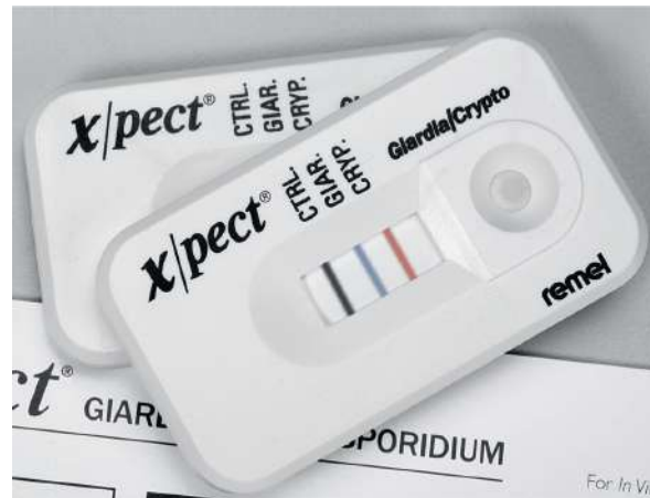
FIGURE 22-3 Remel Xpect ® Giardia/Cryptosporidium immunochromatographic immunoassay. The test uses sample wicking to capture Giardia and Cryptosporidium antigens on discrete test lines containing antigen-specific antibodies for each organism. (Reprinted by permission of Thermo Fisher Scientific, Lenexa, Kansas.)
