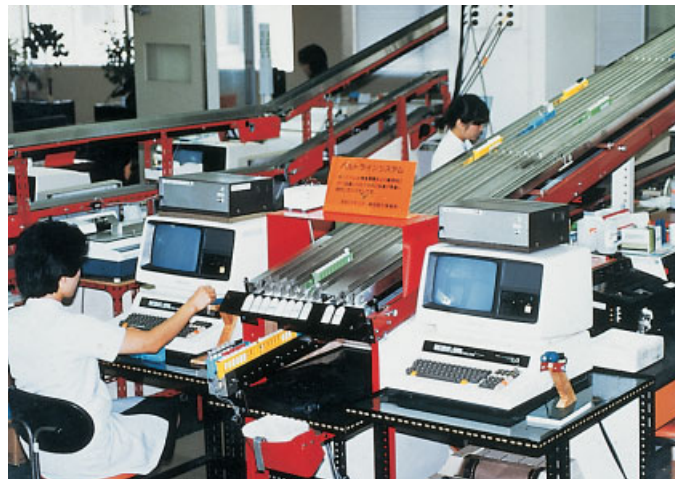
Fig. 19-3 Conveyer belt system to transport samples to robotic analyzers (with kind permission of M. Sasaki, Kochi, Japan)
