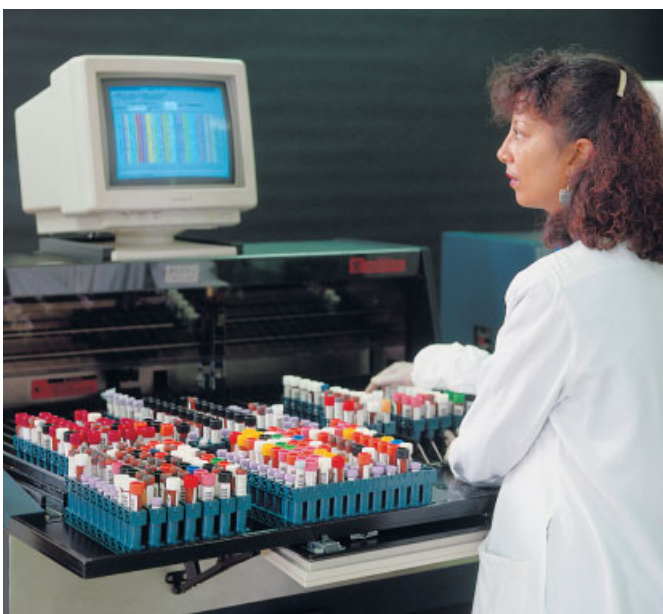
Fig. 19-1 Automated sample sorter system (with kind permission of P. Mountain, Auto-lab, Toronto, Canada)
